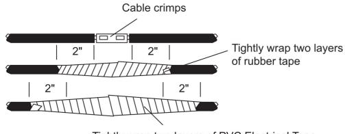
Tightly wrap two layers of PVC Electrical Tape
